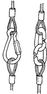
39. Ladders spreaders and wire tethers should be cleaned and inspected for damage after every caving trip, paying particular attention to where the wire rope passes through the rungs or around the swaged eyes. Ladders should preferably be carried in a tackle sack when underground, this prevent them snagging and helps to stop mud being forced into the wire rope.
