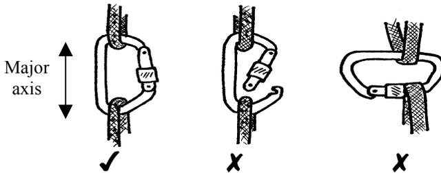
15. Screw gate karabiners should be positioned with the opening part of the gate downwards so that gravity helps to prevent the gate unscrewing. Resist the temptation to give the screw gate a final tighten up when the karabiner is loaded, as it can be very difficult to undo later.
