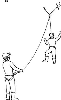
88. When ever possible the pulley or karabiner should be visible from the bottom of the pitch. This will help to reduced friction and prevent twisting and jamming of the ropes. It may be necessary to use a sling or the end of the rigging rope to extend the belay.
