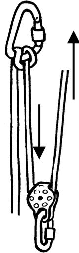
126. **Bell Ringing** When belaying from the bottom the simplest way to assist a tired climber up a pitch is for two or three other cavers to gather around the rope and pull down using their body weight. To prevent the casualty from falling back down the pitch, if all the hauling team happen to let go at the same time, one of cavers at the bottom **MUST** belay the lifeline at all times.
