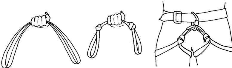
111. To create the harness, hold the sown joint in the one hand with an equally sized loop each side. A knot is then tied in each loop close to and either side of the hand. Depending on the size of the cavers legs either an Overhand, Figure of 8 or Figure of 9 knot should be tied. It is important that the loops are a reasonably good fit around the upper thigh to prevent the loops slipping down and hindering movement
