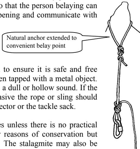
66. The rock must be checked to ensure it is safe and free from cracks, it should “ring” when tapped with a metal object. Do not use the anchor if it makes a dull or hollow sound. If the rock is particularly sharp or abrasive the rope or sling should be protected by using a rope protector or the tackle sack.
