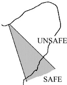
69. If you are using a spike make sure that the sling or rope will not jump off the top when a shock load is applied or released.
