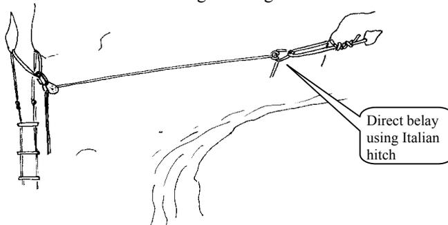
of the ladder it can be used to redirect the rope whilst belaying from the pitch head, but must not be used on its own for the double lifeline. To adequately protect the last person to descend the rope would have to be passed through the pulley/karabiner at the top of the ladder as well as a second pulley/karabiner attached to the main belaying point. This will cause an increase in friction that may make lifelining from the bottom of the pitch difficult.
