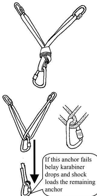
subjected to a shock load as the belay karabiner slides down and then stops at the end of the sling. Because cavers use low stretch ropes this shock load will be very high. If a twist is not placed in the sling the central belay karabiner can slide off the sling if one anchor should fail.
