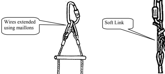
44. **Tethers** These are used to connect a ladder directly to a natural anchor such as a thread, spike or jammed boulder. They have become almost obsolete with the number of artificial anchors available and in most cases a rope or tape sling can be used in their place. However, tethers are especially useful where the limestone is particularly sharp or abrasive and when exploring new caves.
