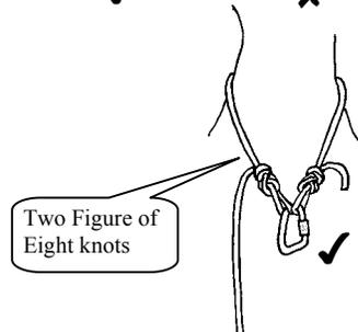
65. The rope can also be used to move the belay point closer to the top of the pitch or climb so that the person belaying can get a better view of what is happening and communicate with the person climbing.
