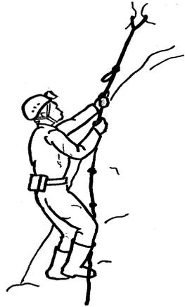
59. It is very difficult to grip a small diameter rope particularly with cold and wet hand. It is beneficial to tie a number of overhand or butterfly knot in the handline to aid grip.
