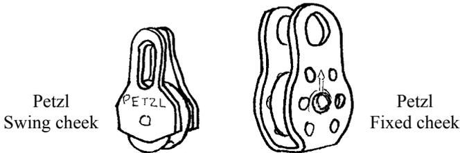
24. The lightweight Petzl swing cheek pulley is designed primarily for tackle hauling and self-rescue. It has a working load of 2kN (200kg) and a minimum (breaking) load of 12kN(1200kg). The lightweight swing cheek is suitable for normal double life lining, but must not be subjected to shock loading or used for heavy load rescues. This is because the entire load is taken on a single small diameter pin.
