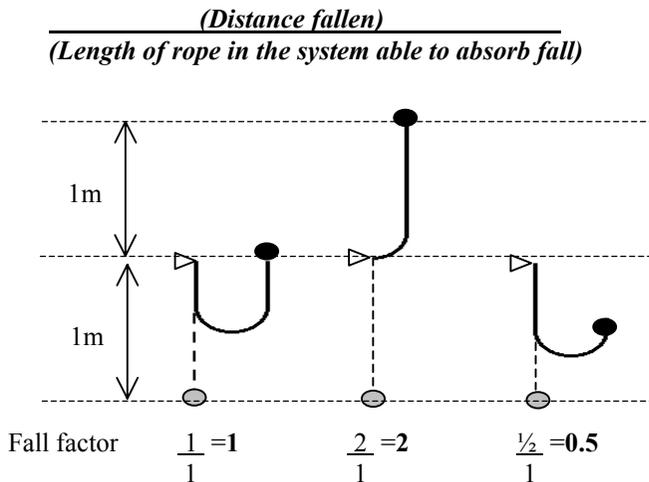
50. Dynamic climbing ropes are designed to stretch and absorb the energy from a large (factor 2) fall and limit the peak force to less than 12kN in order to protect a climber from a fatal shock load. A climbing rope will be rated at the number of factor 1.78 falls it can take before failure occurs. Currently the test is carried out with an 80kg test weight, this is likely to be increased to 100kg. A typical 11mm rope will have a rating of 7-9 falls.
