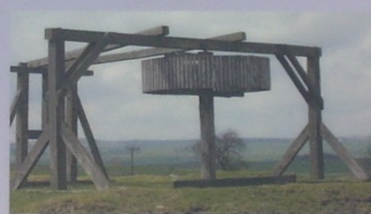
A reconstructed horse-drawn winding gin at Magpie Mine, Sheldon
