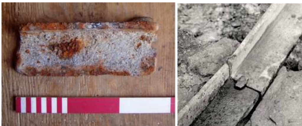
New discovery Plateway with square end and fixing pin slot. Shown in place in right picture.
