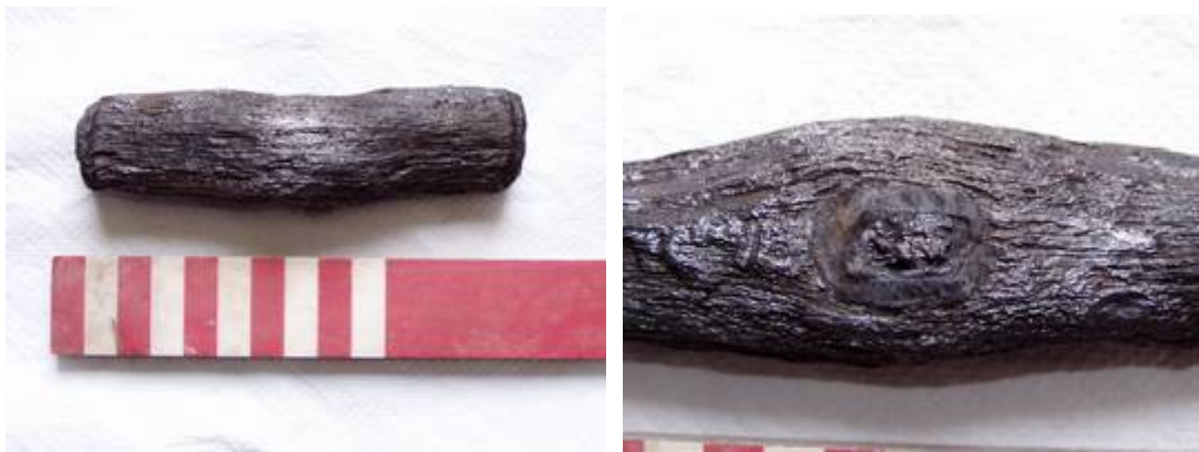
The wrought iron hammer head after electrolysis and drying, and before being treated with tannic acid and coated in red lead and metal paint to prevent air getting to the metal.
