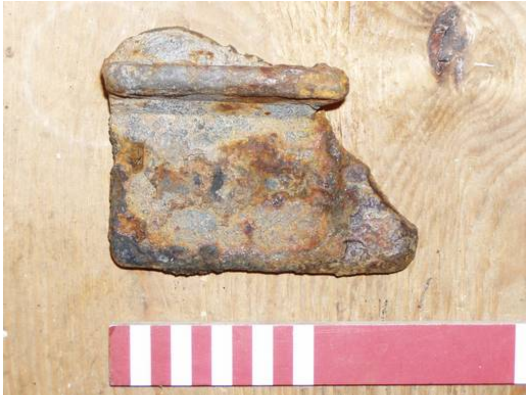
3-inch Plateway with fixing pin slot and larger side seating flange (at the top of the picture).
